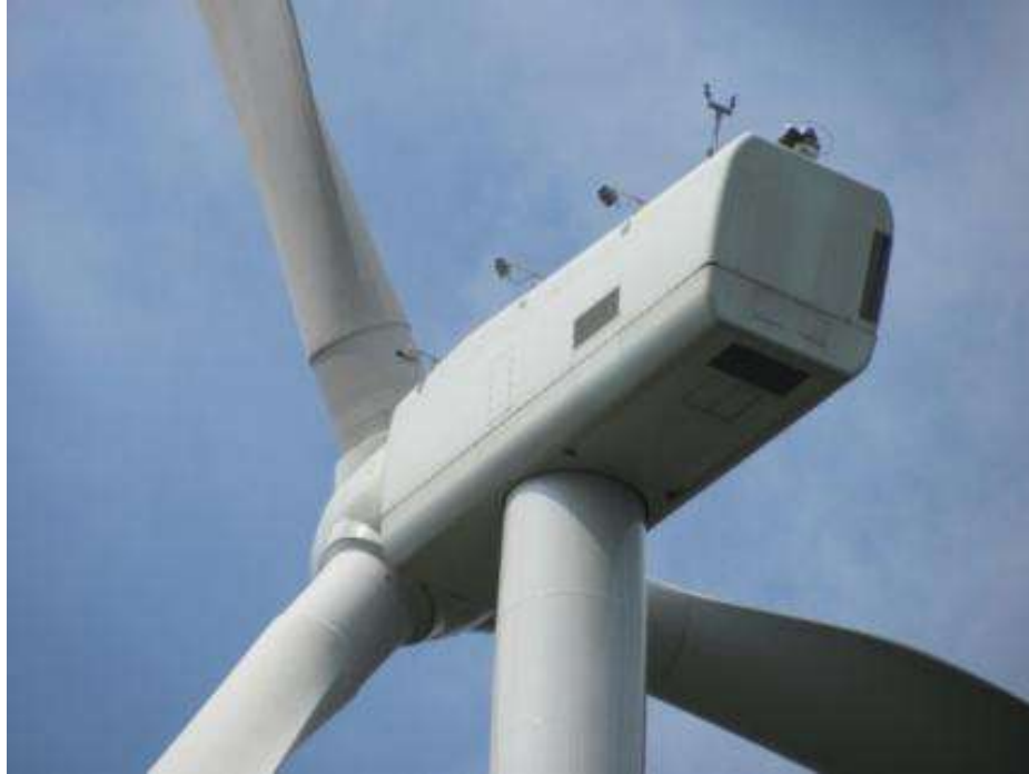
Acoustic deterrent devices mounted on the nacelle of a wind turbine.
