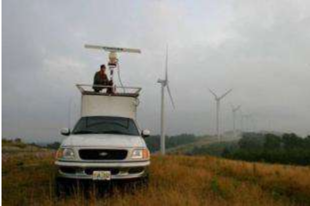
Brian Cooper with ABR, Inc. sets up marine radar to track birds and bats at Mountaineer in West Virginia.
