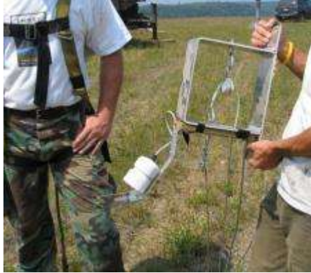
Pulley system for deploying acoustic detector microphones in "bat hats."
