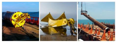
Figure 27 Suction pile anchor, drag embedment anchor and driven pile anchor. *Images courtesy of Acteon, Principle Power and Acteon. All rights reserved.*
