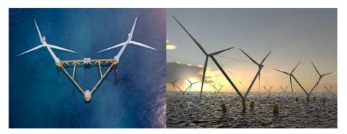
Figure 7 Floating substructures with multiple rotors. *From left to right: Hexicon's TwinWind (image courtesy of Hexicon, all rights reserved) and Aerodyn's Nezzy2 (image courtesy of Aerodyn, all rights reserved).*
