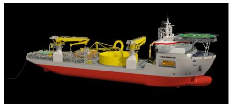
Figure 35 Cable-laying vessel. *Image courtesy of Jan de Nul. All rights reserved.*
