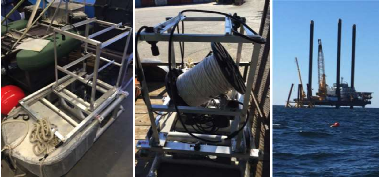
Figure 22. Images of the geosled before deployment (left and center). These two photographs show the tetrahedral array of hydrophones with a spacing of 0.5 m (1.6 ft). Photograph of the surface floats for the sled with WTG 4 in the background (right).
