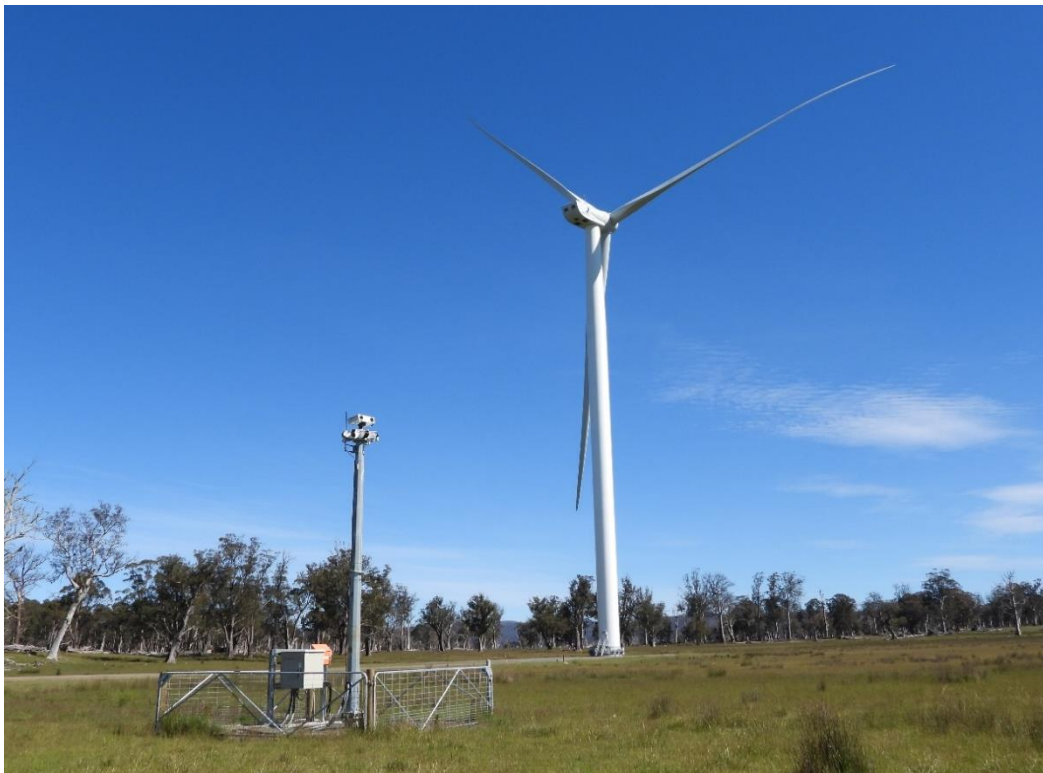
Plate 7: One of the Sixteen IdentiFlight Units installed at Cattle Hill Wind Farm
