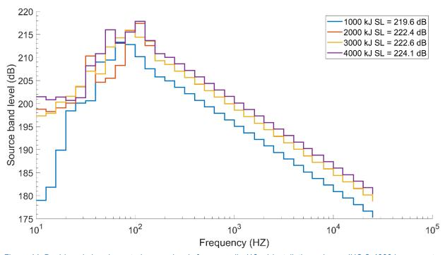
Figure 11. Decidecade band spectral source levels for monopile (12 m) installation using an IHC S-4000 hammer at site L024-114 with a summer sound speed profile.
