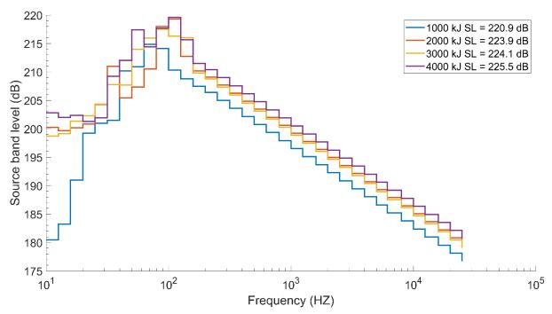
Figure 12. Decidecade band spectral source levels for monopile (12 m) installation using an IHC S-4000 hammer at site L024-114 with a winter sound speed profile.
