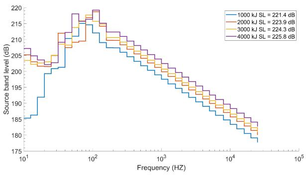
Figure 10. Decidecade band spectral source levels for monopile (12 m) installation using an IHC S-4000 hammer at site L024-002 with a winter sound speed profile.
