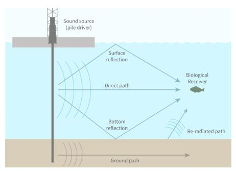
Figure 3. Sound propagation paths associated with impact pile driving (adapted from Buehler et al. 2015).
