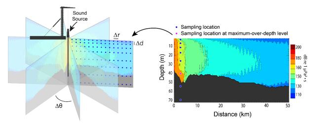
Figure G-2. Modeled three-dimensional sound field (N×2-D method) and maximum-over-depth modeling approach. Sampling locations are shown as blue dots on both figures. On the right panel, the pink dot represents the sampling location where the sound level is maximum over the water column. This maximum-over-depth level is used in calculating distances to sound level thresholds for some marine animals.
