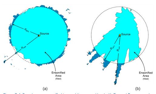
Figure G-4. Sample areas ensonified to an arbitrary sound level with  $R_{\text{max}}$  and  $R_{95\%}$  ranges shown for two different scenarios. (a) Largely symmetric sound level contour with small protrusions. (b) Strongly asymmetric sound level contour with long protrusions. Light blue indicates the ensonified areas bounded by  $R_{95\%}$ ; darker blue indicates the areas outside this boundary which determine  $R_{\text{max}}$ .
