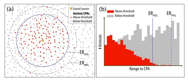
Figure 5. Example distribution of animat closest points of approach (CPAs). Panel (a) shows the horizontal distribution of animats near a sound source. Panel (b) shows a stacked bar plot of the distribution of ranges to animat CPAs. The 95% and 99% Exposure Ranges (ER<sub>95%</sub> and ER<sub>99%</sub>) are indicated in both panels.
