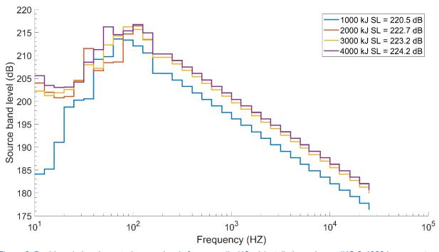
Figure 9. Decidecade band spectral source levels for monopile (12 m) installation using an IHC S-4000 hammer at site L024-002 with a summer sound speed profile.
