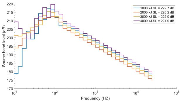
Figure 13. Decidecade band spectral source levels for monopile (15 m) installation using an IHC S-4000 hammer with a summer sound speed profile.
