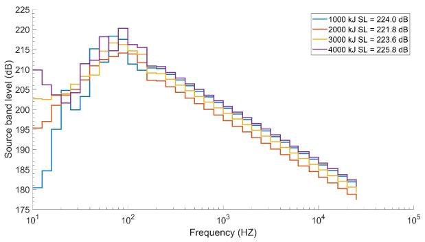
Figure 14. Decidecade band spectral source levels for monopile (15 m) installation using an IHC S-4000 hammer with a winter sound speed profile.
