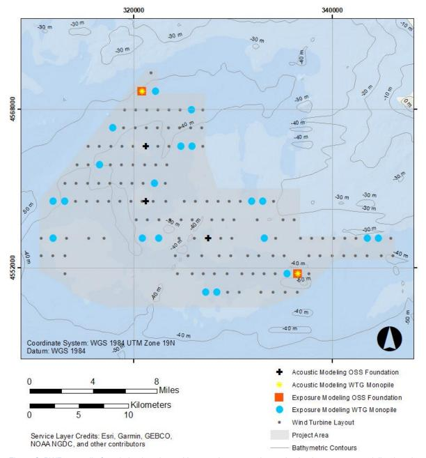
Figure 2. RWF monopile foundation locations with acoustic propagation and animal movement modeling locations.
