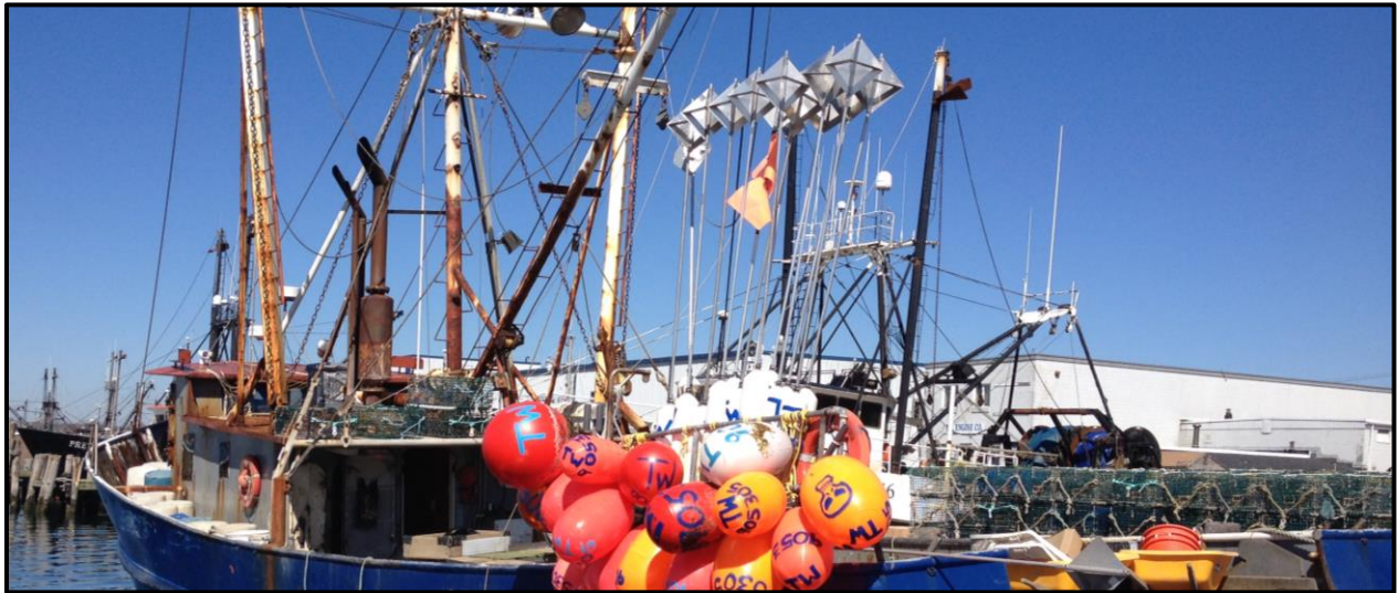
Figure 2.7: Example of pot vessel with buoys and highflyers stored on vessel deck
