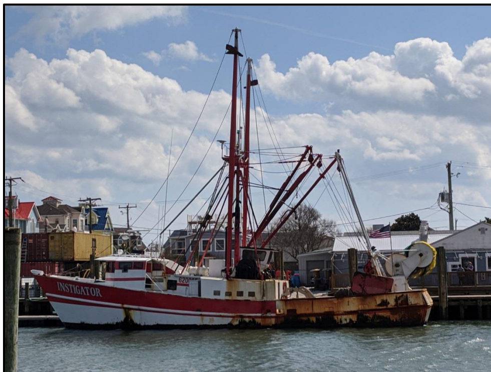
Figure 2.4: The fishing trawler Instigator delivers her catch in Ocean City MD. Typical otter board trawl doors can be seen shipped near the vessel stern. (Photo: Wolfgang Rain/Sea Risk Solutions).
