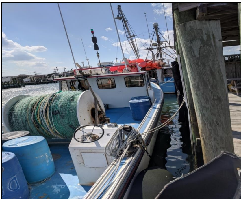
Figure 2.13: Deck of gillnet vessel with net reel loaded for black sea bass fishing.
