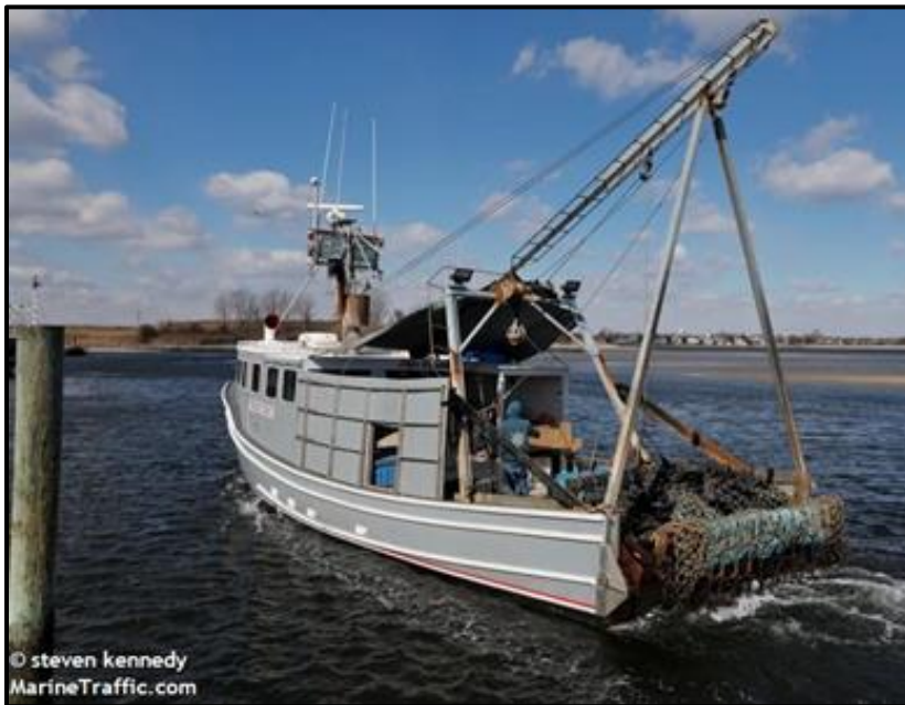
Figure 2.26: Example of a day boat scallop vessel working a single dredge
