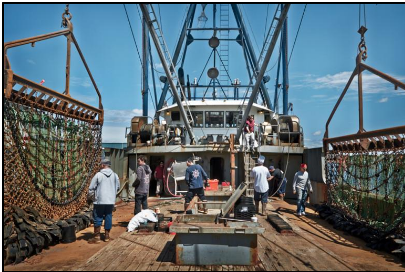
Figure 2.25: Scallop dredges suspended on the deck of the vessel; chain mesh is designed to keep rocks/boulders from entering the dredge.
