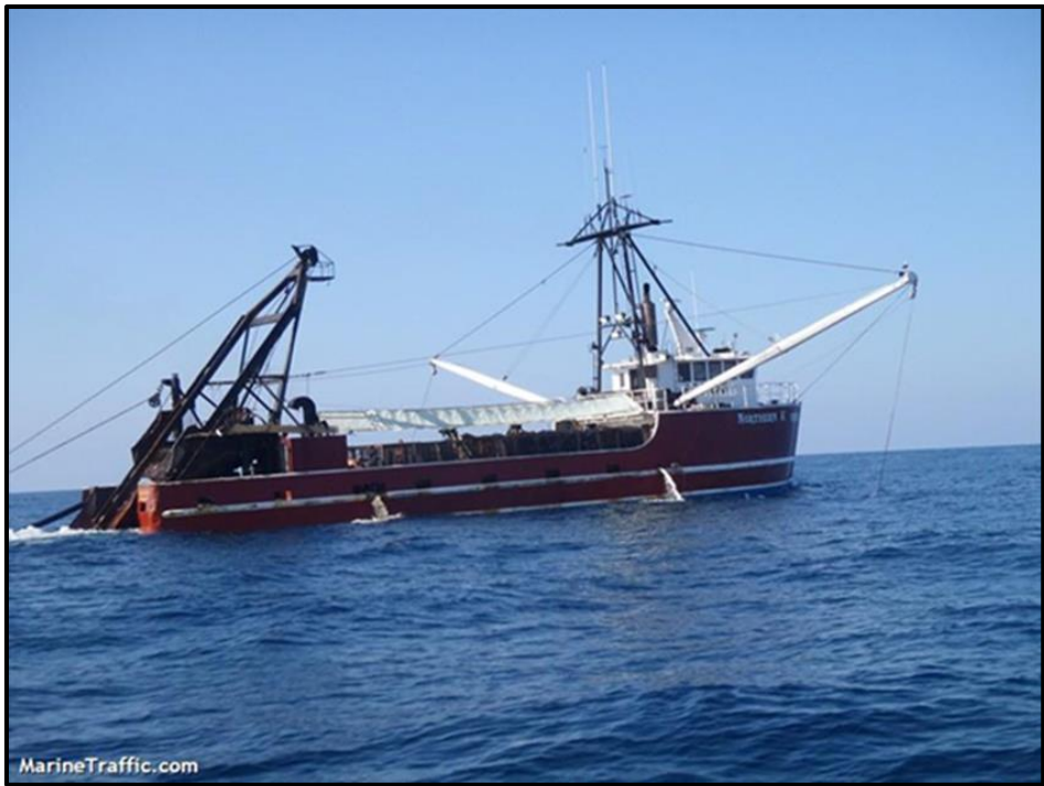
Figure 2.18 Hydraulic clam dredge fishing vessel in operation
