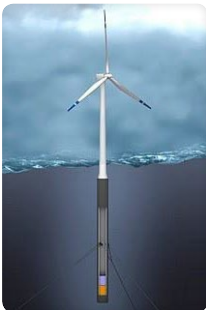
Floating Wind Turbine Concept (Mitchell, 2009)
