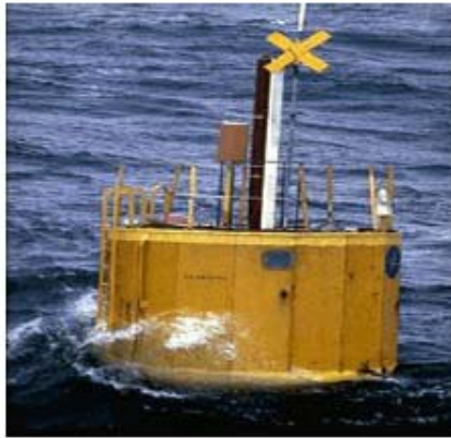
FIGURE 5 AquaBuOY Point Absorber Wave Energy Converter (Source: AquaEnergy Group, Ltd. 2005)
