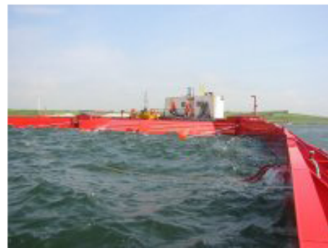
FIGURE 6 Wave Dragon Overtopping Device (Source: Wave Dragon 2005)
